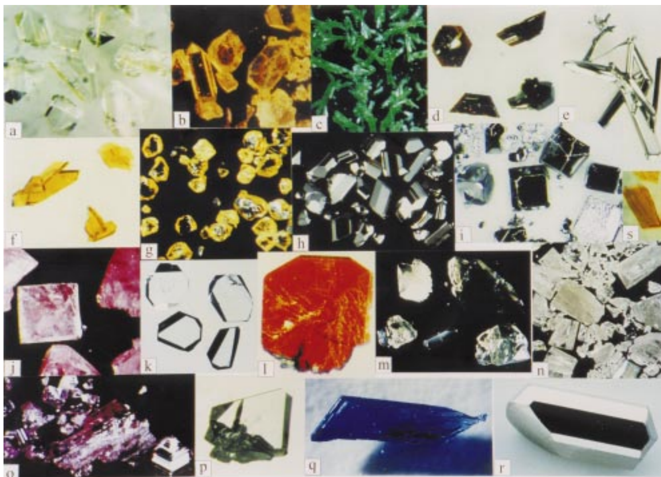
Abbildung 5. Durch chemischen Transport erhaltene Kristalle: a) \text{Yb}_2\text{Si}_2\text{O}_7 (Kristallgröße ca. 2 mm), b) \text{NiSO}_4 (0.5 mm), c) \text{Pr}_2\text{Ti}_3\text{O}_8\text{Cl}_2 (0.3 mm), d) \text{RhPO}_4 (0.5 mm), e) \beta\text{-WP}_2 (5 mm), f) \text{Rh}(\text{PO}_3)_3 (0.4 mm), g) \text{Sm}_2\text{Ti}_2\text{O}_7 (0.3 mm), h) \text{CoP}_2 (2 mm), i) \text{CoP}_3 (2 mm), j) \text{NdNbO}_4 (1 mm), k) \text{CuSO}_4 (0.5 mm), l) \text{Pd}_2\text{P}_2\text{O}_7 (2 mm), m) \text{FeSO}_4 (1 mm), n) \text{Ta}_2\text{O}_5 (0.4 mm), o) \text{Nd}_4\text{Ti}_9\text{O}_{24} (1 mm), p) \text{CuP}_4\text{O}_{11} (4 mm), q) \text{Cr}_2\text{P}_2\text{O}_7 (10 mm), r) \text{CrP} (8 mm), s) \text{Ce}_2\text{Ti}_3\text{O}_8\text{Cl}_2 (0.5 mm).
